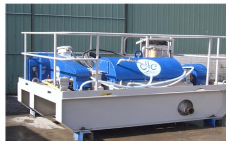
The Centrifuge will be mounted on the dewatering unit, high enough to allow the effluent to gravity feed to the dilution/clean water tank, and to allow the solids discharges to fall into the collection area or centrifuge auger. This centrifuge will be located on a stand next to the pits and the active system centrifuge(s).
